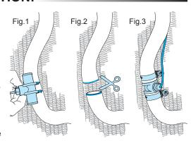
Radiator Hose Temperature Sensor 1: Mark hose, 2: Cut Hose, 3: Install Sensor
